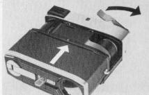
Rotiere rapid-advance lever until film is advanced by take-up drum and is tightly stretched. Replace camera back, push it upward as far as possible and lock, fig. 6.
