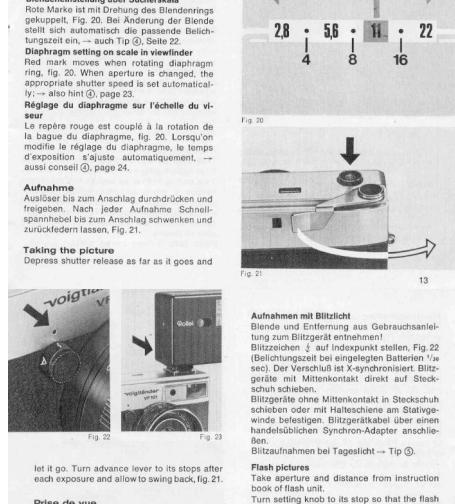
tached with a flash bracket to the tripod socket. Connect flash cable by means of a standard sync-adapter.
